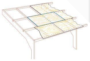
• The installation is carried out on perimeter supports. The panels are laid on a continuous support on their 4 sides and on at least an intermediate one. As a result a double square design is obtained. The minimum supporting width at each end of the panels should be at least 20 mm.
