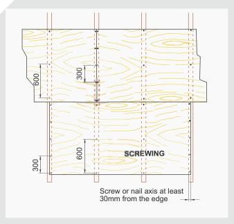
• The length of the screws should allow the thread to overdrive the wing of the steel profile by around 5 mm. When using self-drilling tapping screws, the fixings on THEBAULT plywood panels should take place at least 10 mm away from their supported edges.
